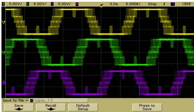
Fig.23: PSC-SFO PWM output voltage (Modulation index 1.1)
