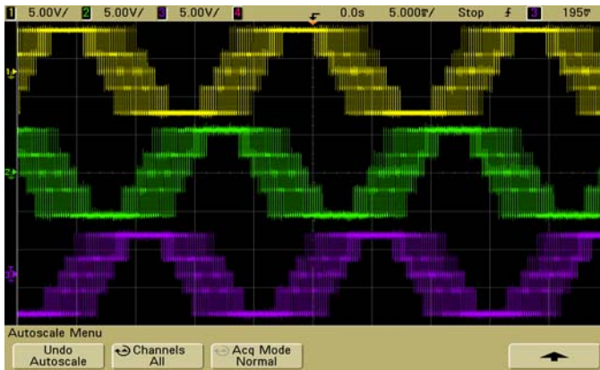
Fig.20: PSC PWM output voltage (Modulation index 1.1)
