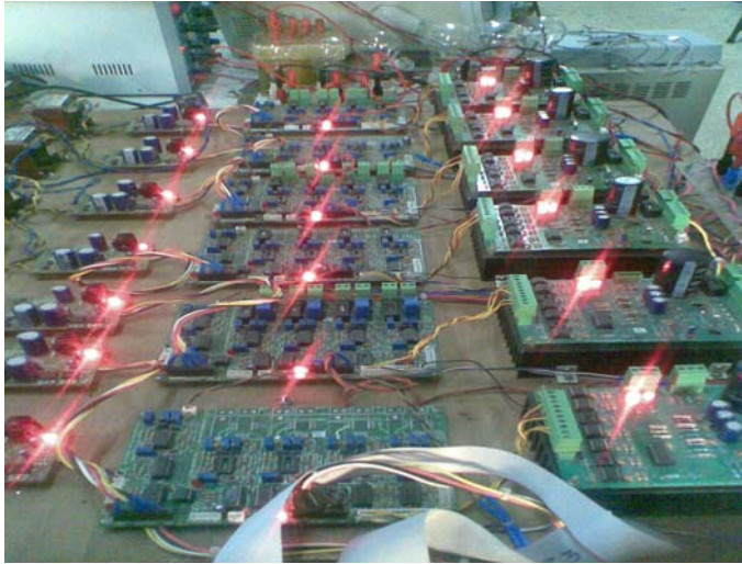
Fig.25: Hardware setup of three phase cascaded multilevel inverter
