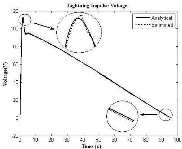
Figure. 7 Comparison of analytical and estimated values of lightning impulse voltage using PSO - WNN
