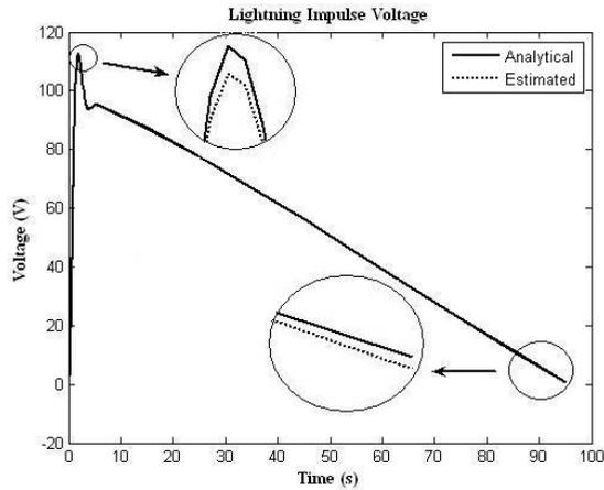
Figure. 4 Comparison of analytical and estimated values of lightning impulse voltage using WNN
