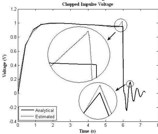
Figure. 6 Comparison of analytical and estimated values of chopped impulse voltage using WNN
