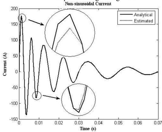
Figure. 5 Comparison of analytical and estimated values of non-sinusoidal current using WNN
