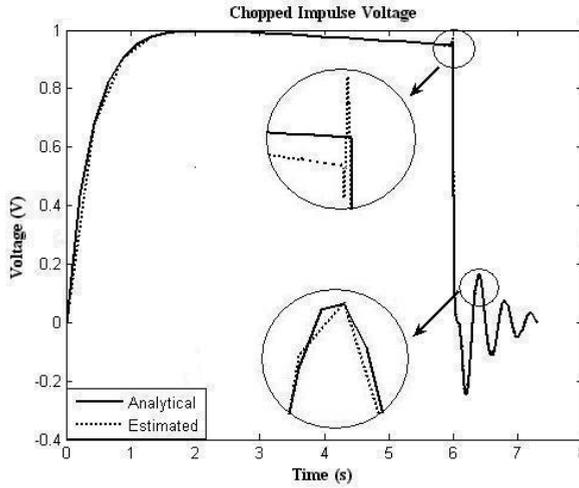
Figure. 9 Comparison of analytical and estimated values of chopped impulse voltage using PSO – WNN
