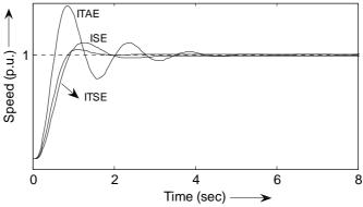
Figure 8. Comparison of gas turbine plant response with PID controller, tuned using ISE, ITAE and ITSE.
