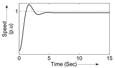
Figure 3. Response of gas turbine plant without secondary controller
