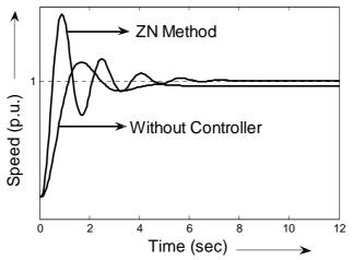
Figure 4. Response of gas turbine plant without controller and with PID controller tuning using ZN method - A Comparison.
