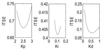
Figure 6. Performance index ITAE of gas turbine plant
