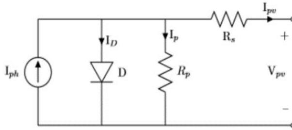
Fig. 2. Single diode Model
