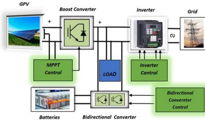
Fig. 1. System description block diagram
