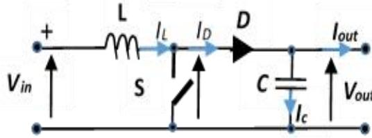
Fig. 5. Electrical circuit of the Boost converter
