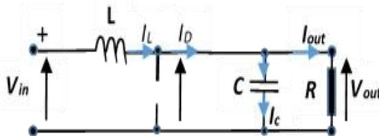
Fig. 7. Electrical Circuit when S is opened
