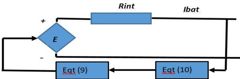
Fig. 9. Circuit diagram of battery
