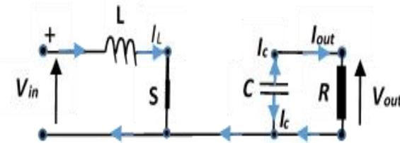
Fig. 6. Electrical Circuit when S is closed
