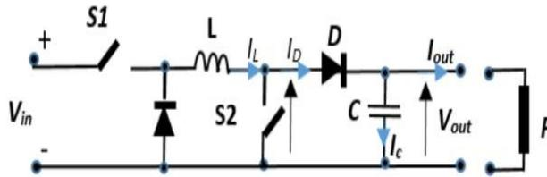
Fig. 8. Electrical Circuit of Buck-Boost converter
