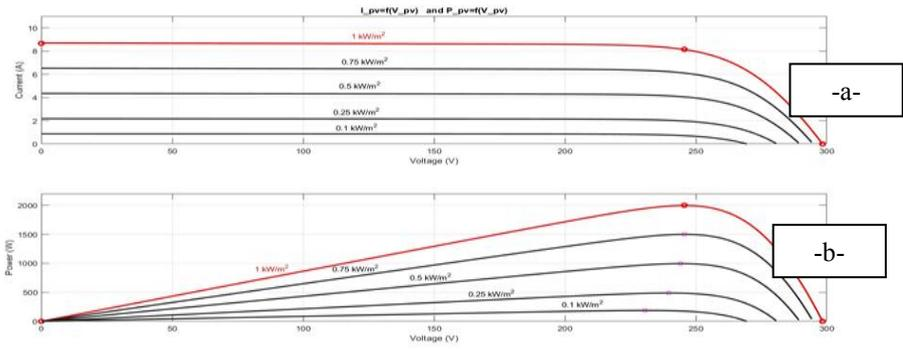
Fig. 3.  $I_{pv}=f(V_{pv})$  and  $P_{pv}=f(V_{pv})$  where  $E$ =variable and  $T$ =Cont= $25^{\circ}C$
