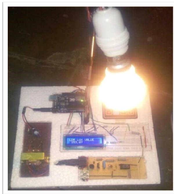
Fig. 7. The actual circuit configuration of the Lux Adjuster Controller for Solitary Ocular Comfort
