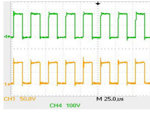
Fig. 20. The voltage stress on S_1 (channel 10) and S_2 (channel 4) during step-up operation of the converter.
