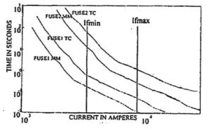
Fig. 2. Fuse-fuse coordination area (CA) [10]
