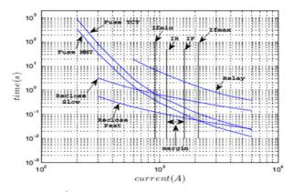
Fig 3. Recloser-fuse-relay CA
