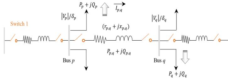
Fig. 1. Example distribution line between bus  $p$  and bus  $q$  in presence switches device
