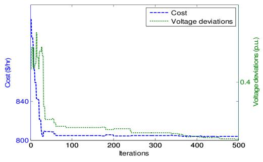
Figure.3 Variations of fuel cost and voltage deviations for Case 2.
