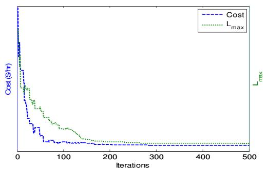
**Figure.4** Variations of fuel cost and stability index for Case 3. Table 4: Comparison of *Lmax* index obtained with different algorithms.
