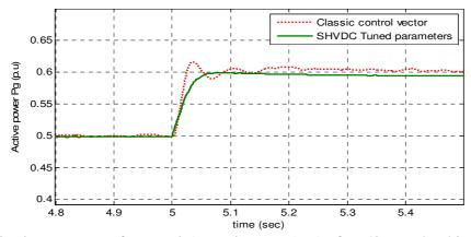
Fig. 9. Response of  $P_g$  to +0.1 step in  $P_{g_ref}$  (p.u) after 50 MW load increase
