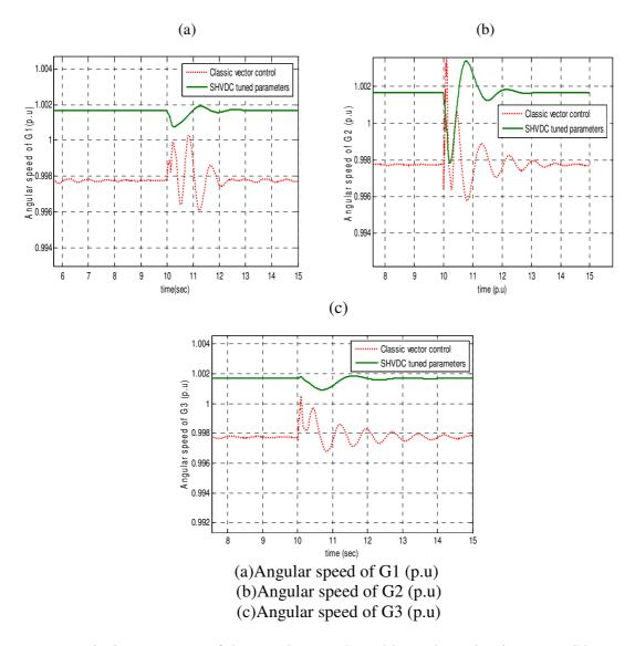
Fig.8. Responses of the angular speed to 100 ms short circuit near to G2
