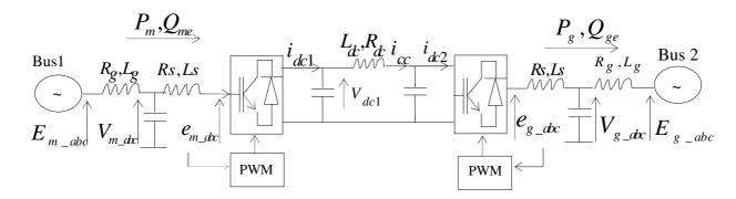
Fig. 2. Two terminal VSC-HVDC link
