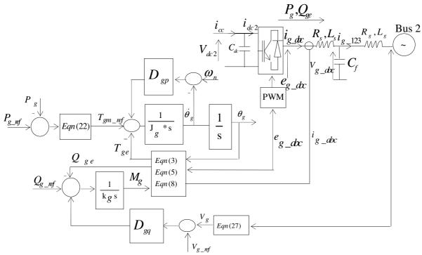
Fig. 3. Model of the synchronverter: power and electronic parts [17]
