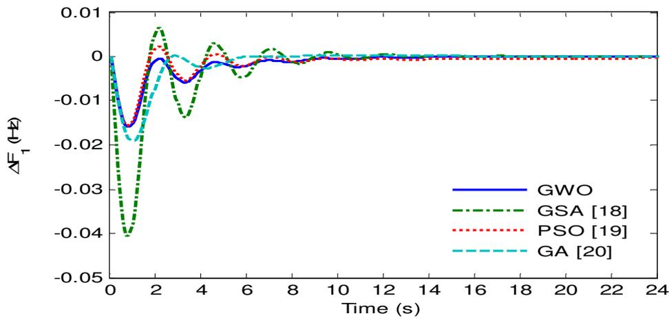
Figure 6(a) Change in frequency of area 1 on -25% load change in area-1
