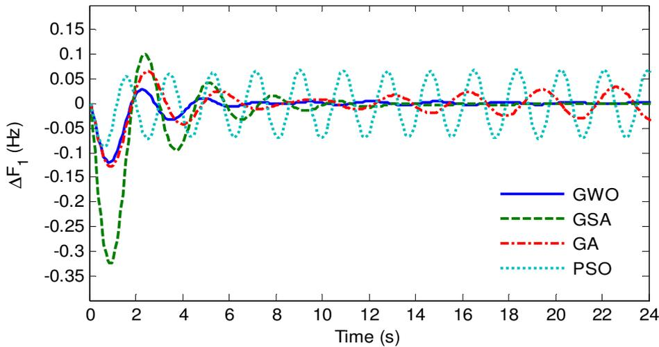
Figure 7 Change in frequency of area 1 by 25% load through J2.
