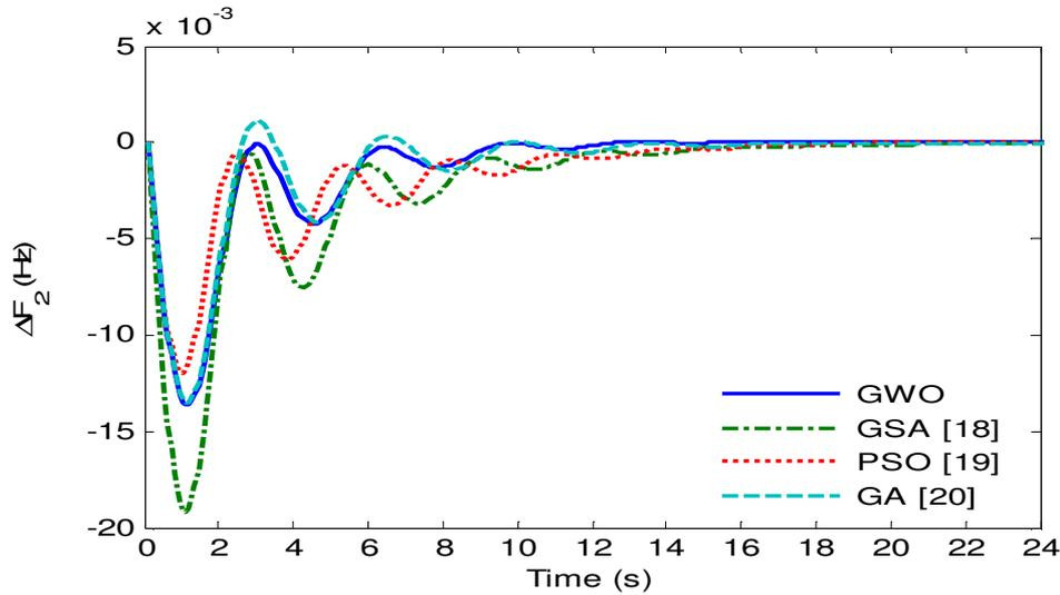
Figure 5(b). Change in frequency of area 2 on +25% load change in area-1
