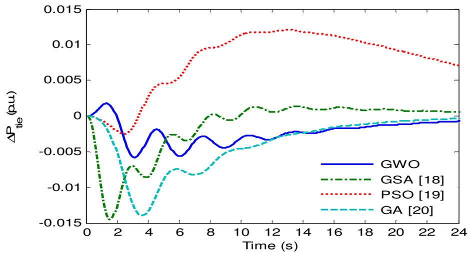
Figure 3(c). Change in tie line power by +10% load change in area-1
