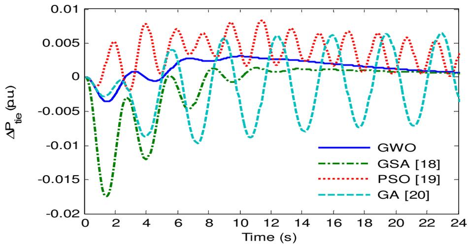
Figure 4(c). Change in tie line power by +20% load change in area-2
