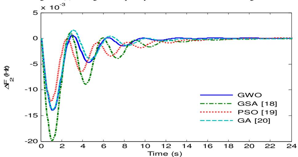
Figure 6(b) Change in frequency of area 2 on -25% load change in area-1
