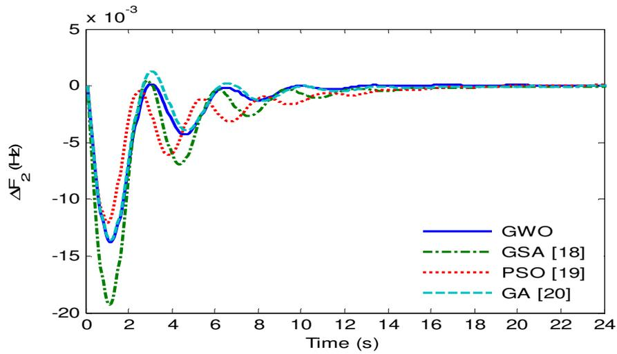
Figure 3(b). Change in frequency of area 2 by 10% load change in area-1
