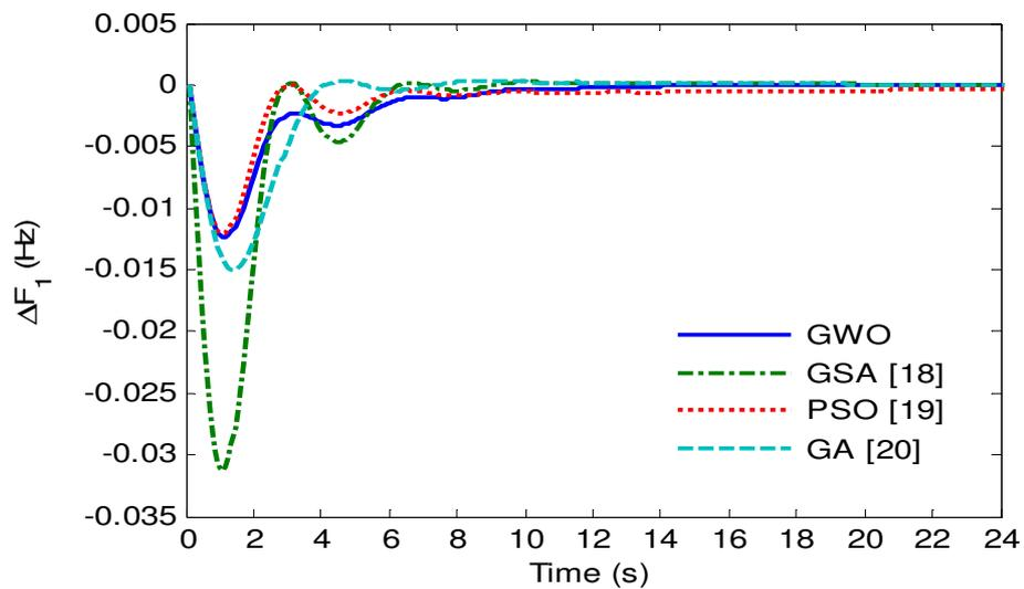
Figure 5(a). Change in frequency of area 1 with 25% increase in load in area-1
