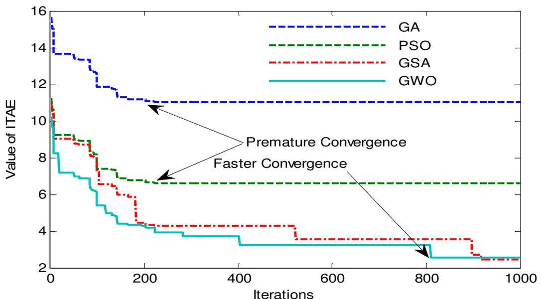
Figure 8 Convergence Characteristics of Proposed GWO Regulators
