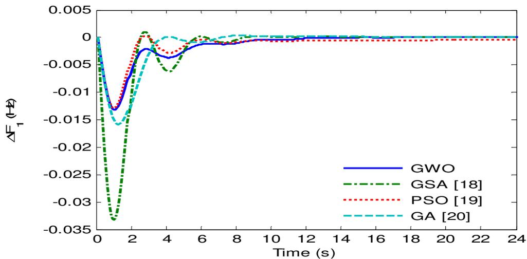
Figure 3(a). Change in frequency of area 1 by 10% load change in area-1
