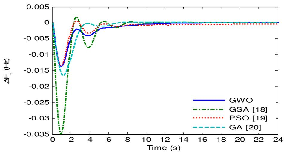
Figure 4(a). Change in frequency of area 1 by +20% load change in area-2
