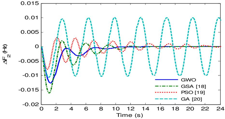
Figure 4(b). Change in frequency of area 2 by +20% load change in area-2
