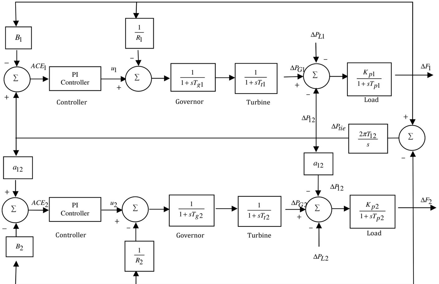
Figure 1 Transfer function model of two area non reheat thermal power system.
